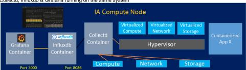
2. Collectd running on the compute node and Influxdb & grafana running on the controller node
